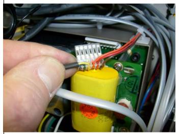
Note how the standoff slides over the hex head nuts. It is easy for the standoffs to slip off when you are installing the new circuit boards.
