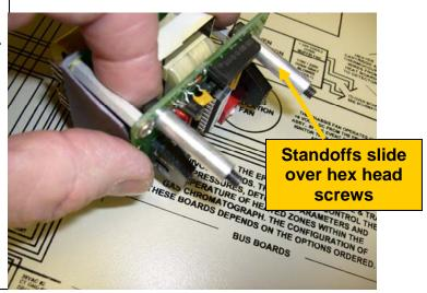
Install the new circuit board set. It is helpful to tilt the board slightly so the standoffs don't fall off while you are wiggling the boards into position.
