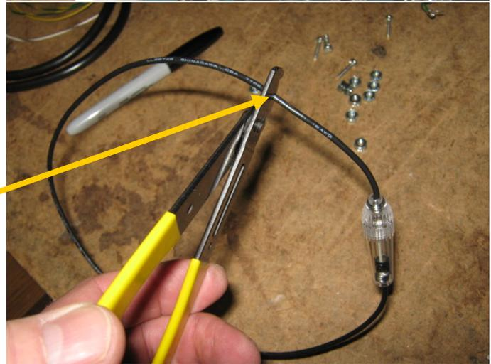
Crimp the longer side of the fuseholder wire to a ring terminal and then fasten to Terminal#2
