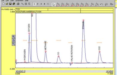
The same instrument produced this chromatogram, separating a sample mix of 1% fixed gas standard and ethane. With the built-in PeakSimple data system, the gas sampling valve was programmed to inject the sample loop contents into the carrier gas stream at 5 seconds, then rotate back at 6 minutes, after CO elution.
