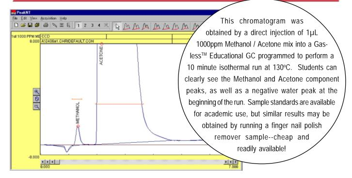
The CCD detector responds to all hydrocarbons at a detection limit of 100ppm. Hayesep-D packed columns are useful for analyzing gases and low molecular weight compounds such as alcohols, aldehydes, and ketones. Inexpensive samples are available at grocery, drug, and
