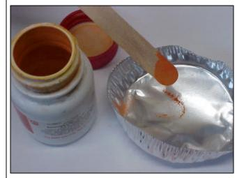
8 Roll a bit of the quartz wool into a cigar shaped plug and coat it with the HgO powder. Insert the plug into the blank reaction tube. Optionally insert another plug of un-coated quartz wool after.
