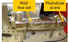
covered with aluminized silicone foam insulation and must be hot enough to keep the gaseous mercury vapor liberated from the mercuric oxide from condensing.
