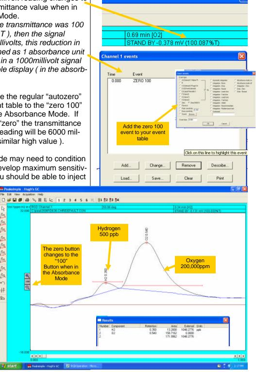
on an appropriate column (typically 2 meter molecular sieve 5A) and see ambient hydrogen at 500ppb similar to the chromatogram shown.
