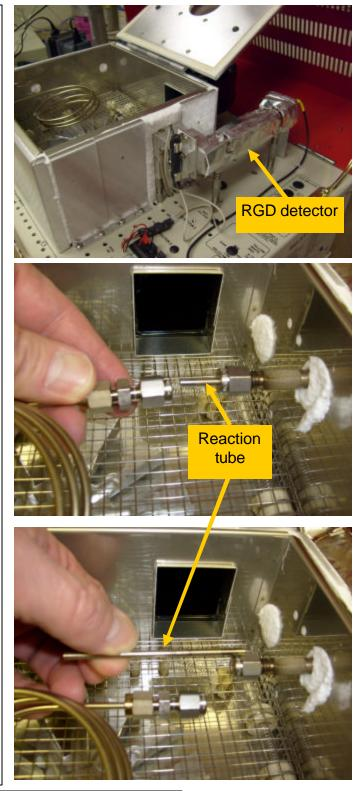
The reaction tube has a 20 micron pore size stainless steel frit on the downstream end. Mercuric Oxide suspended on quartz (fused silica) wool is placed into the open end of the reaction tube.
