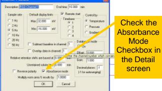
Notice that the millivolt reading changes to include the transmittance value when in the Absorbance Mode.
