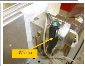
Note that the millivolt reading should increase from a number close to zero (0.00 millivolts) to some larger number when the UV lamp is turned on. This larger number is the **transmittance** (100% T). Ideally this number is greater than 100 millivolts but the actual number will vary as the Mercuric Oxide in the reaction tube becomes conditioned.
