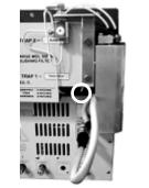
The spring tail (encircled in white) protrudes from the bottom of the front valve oven duct.
