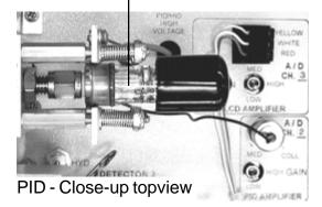
display button on the front control panel. The sensitivity of the lamp increases proportionally to the current applied, but operation at higher currents reduces lamp life. The PID operating current range is 70-125. A setting of 70 should provide the user with sufficient sensitivity and lamp durability. Most PID applications can be performed using LOW gain.
