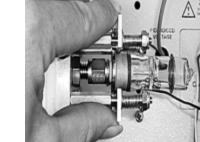
The collector electrode protrudes into the cell
