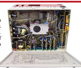
6. Unplug the fan, and unscrew the four screws to remove the aluminum shield so you can pull out the old fan motor (leave the black rubber grommets in the GC chassis). Cut the two black wires that provide power to the motor (crimp connectors are provided to connect the new motor to the black power wires).
