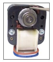
6. Use your SRI screwdriver to pry the bearing/armature assembly from the fan motor.
