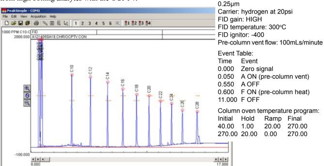
This chromatogram is from the same GC. It was made with the same analytical parameters, except a slightly different event table was used. In this event table, the pre-column heat was not kept on long enough to transfer the highest boiling analytes to the analytical column. The last three peaks are broad
