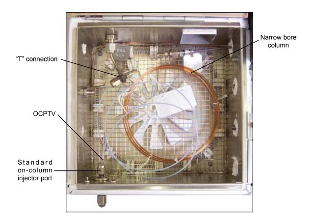
Like the Split/Splitless injector, the OCPTV has a split vent and needle valve for venting solvent while concentrating sample.
