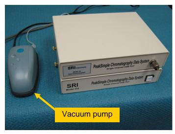
The SRI Instruments Model 30 Gas Chromatograph is a simple low cost system intended for basic GC applications such as measuring Hydrogen in Air or alcohol in water. The extremely small size, USB connection to any Windows computer (laptop) and ability to operate on room air using the included vacuum pump makes the Model 30 perfect for field operations. Helium carrier gas may also be used with the optional carrier gas pressure regulator kit.
