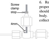
6. Replace the electrodes and check for proper alignment. The collector electrode should extend about 4mm into the detector body. An existing screw clamp stop on the collector electrode should allow replacement without readjustment. Should adjustment be required, loosen the screw clamp to position the electrode, then tighten it to hold the position. To position the arc
