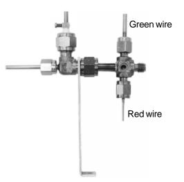
electrodes can develop a coating of soot, which can cause the arc to flicker or change position, resulting in sudden baseline jumps.
