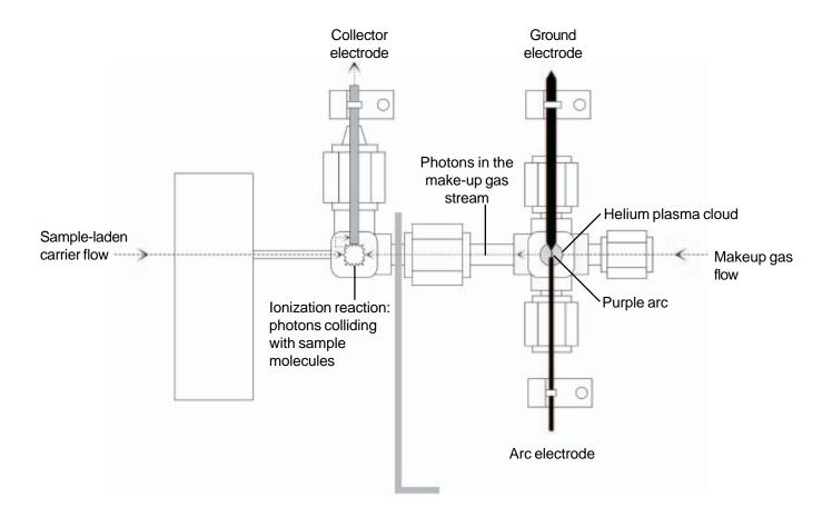
NOTE: If the arc electrode is covered with Teflon<sup>TM</sup> (translucent) insulation, it should leave 1mm of its tip exposed. If the flat electrode is covered with ceramic (white) insulation, then the tip should be flush with the edge of the insulation sleeve. There should be a 1-2mm gap between the arc electrodes, and this gap should be centered in the arc cross.
