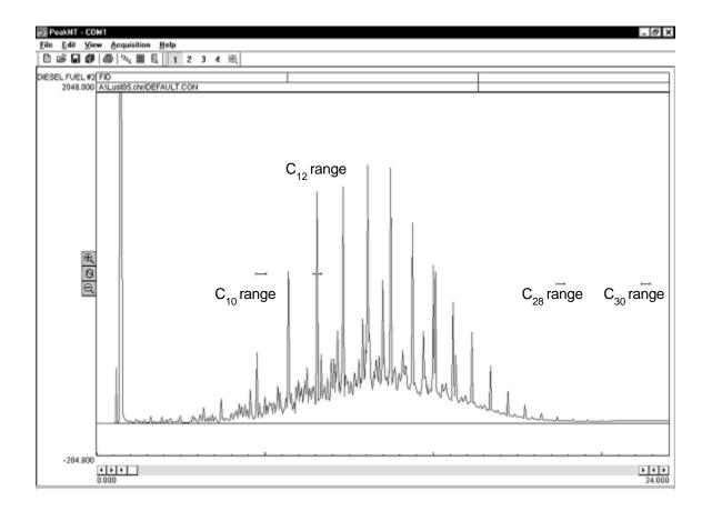
Sample: diesel fuel #2 Method: direct injection Column: 60m MXT-VOL Carrier: helium @ 10mL/min FID gain: HIGH FID temp: 325°C FID ignitor: -400
