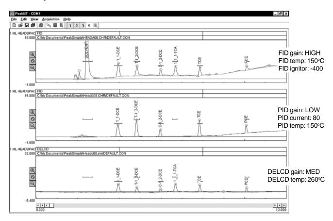
Sample: 1mL headspace from 50ppb Japanese standard in water Method: manual headspace injection Column: 60m MXT-VOL Carrier: helium @ 10mL/min
