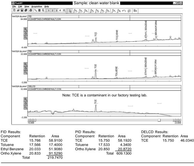
Determine the carryover level by comparing the areas of the two PID Toluene peaks resulting from the sample and blank runs:  $\frac{4}{353} = \frac{x}{10ppb}$ 353x = 40ppbx = 0.1133ppb
