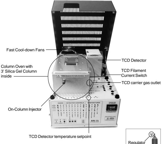
The TCD Detector is located inside its own oven, mounted on the right rear of the Column Oven as shown above. Its temperature is factory preset at 100°C, but it may be heated up to 130°C by adjusting the trimpot with the small blade screwdriver attached to the front right corner of your GC. The trimpot looks like a small brass screw and is located inside the labeled hole on the top edge of the front control panel.
