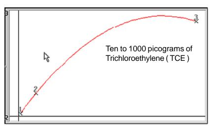
DELCD linearity in high sensitivity mode is shown at right from 10 to 1000 picograms (10-1000PPB).
