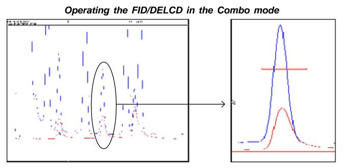
DELCD peak overlaid on FID peak for PCE, then expanded for clarity. The smaller peak is the DELCD response.
