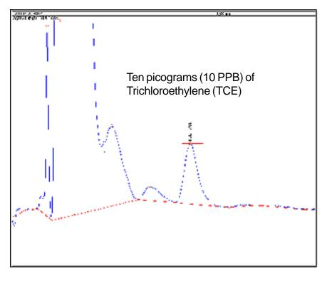
Operating the FID/DELCD in the high sensitivity DELCD only mode
